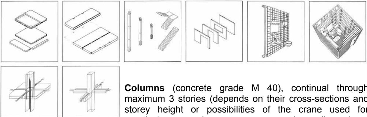
**Columns** (concrete grade M 40), continual through maximum 3 stories (depends on their cross-sections and storey height or possibilities of the crane used for erection), possessing square cross-section – dimensions: 30 x 30 – 60 x 60 cm.
